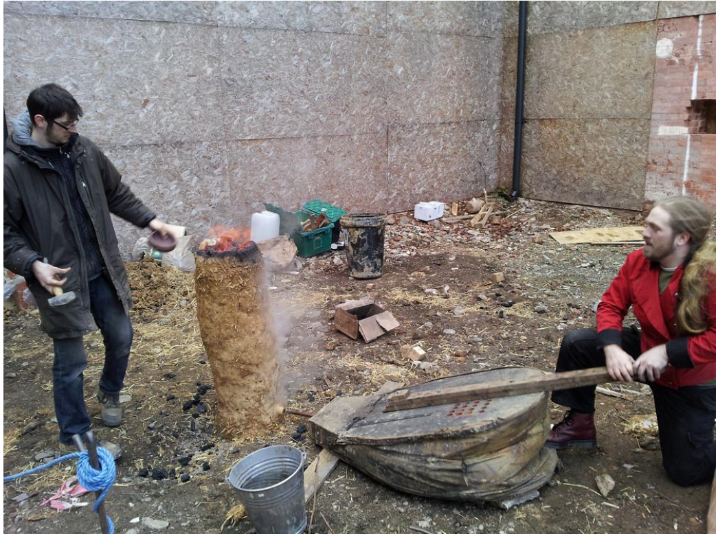
Figure 6.7: Making iron in a clay foundry at The Telling 2013. Own photo.
